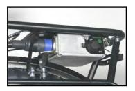
Insert two countersink screws through the countersunk holes in the top of the luggage carrier and through the lugs on the left and right of the control unit.
