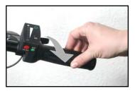
on 36V The system must be switched off to start with! To check the automatic return, twist the twist grip backwards and then release (see photo). The twist grip must immediately return to its initial (zero) position.
