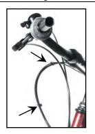
Tie the twist grip cable and the brake and gear cables together with cable ties or coiled cable. Make sure that the cables do not restrict handlebar lock-to-lock movement.
