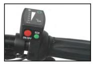
The twist grip incorporates a display and operating unit with a number of pushbuttons and light-emitting diodes (LEDs).
