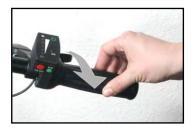
Remove the handlebar grips.
