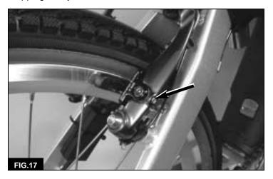
Small changes in the modulation adjustment can have a significant effect upon brake pressure and stopping ability. Whenever you adjust the modulation, adjust each caliper in 1/4 turn increments and test the brakes. Always adjust each side of the brakes equally. If you increase the modulation on the left caliper by 1/4 turn, you should also increase the modulation on the right caliper by an equal amount.
