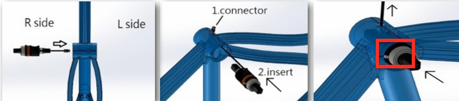
1. Simply insert the torque sensor into the bottom bracket as in the photos from bike right side to bike left side.
