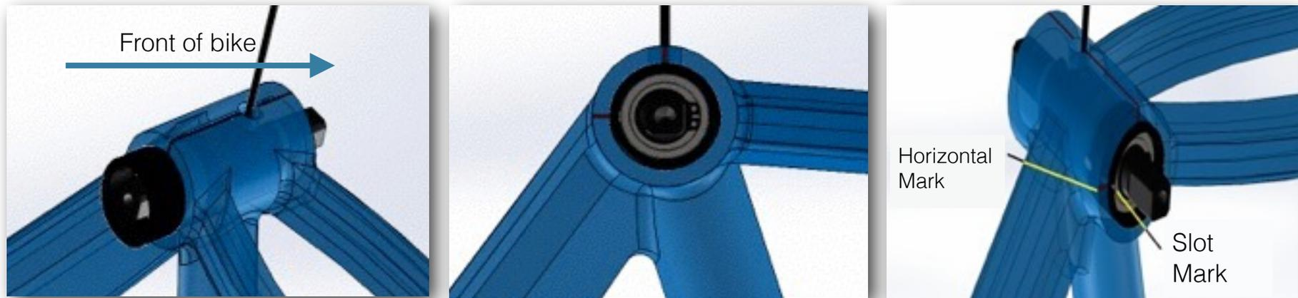
1. Use a light coating of grease on the treads of the Right Side Adjusting Cup.
