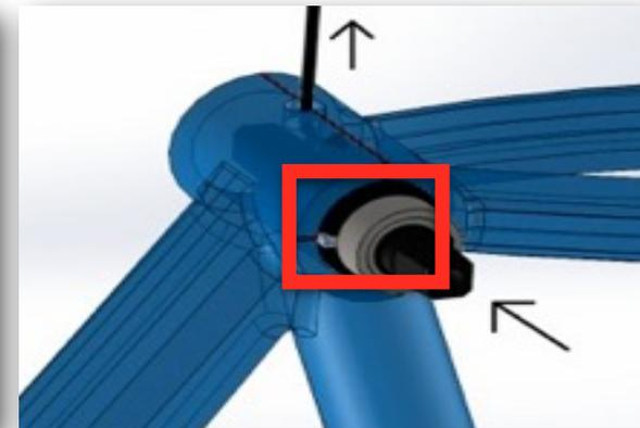
1. Simply insert the torque sensor into the bottom bracket as in the photos from bike right side to bike left side.
