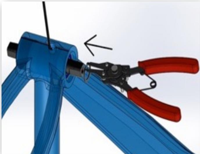
1. Insert rotor bearing into position
