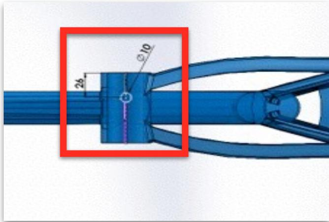
For easy installation and reduced risk of damage to the cable it is important the BB shell has a hole 26mm from the left side of the frame. For the standard connection connector a 10mm diameter hole is recommended.
