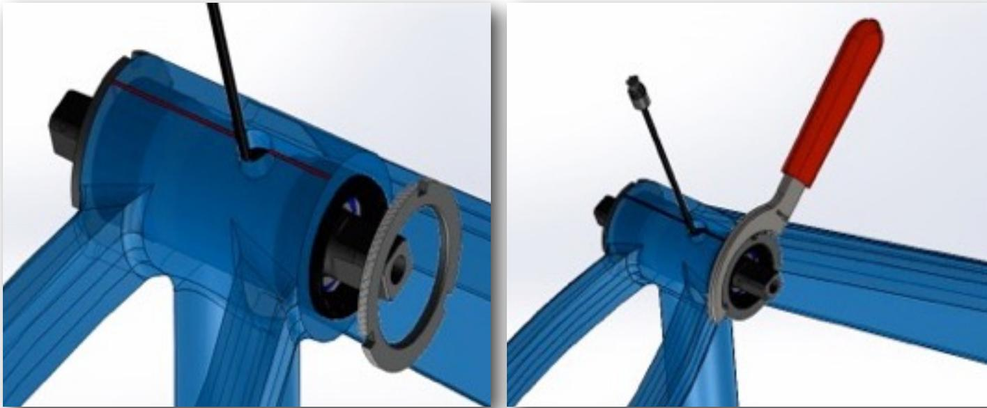
1. Tighten left side lock ring onto cup and tighten until it is secure against bottom bracket shell. Repeat for the right side.
