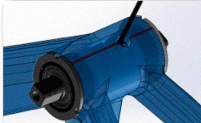
1. Install the rubber dust seal from by sliding it over the Torque Sensor Shaft from the right side.
