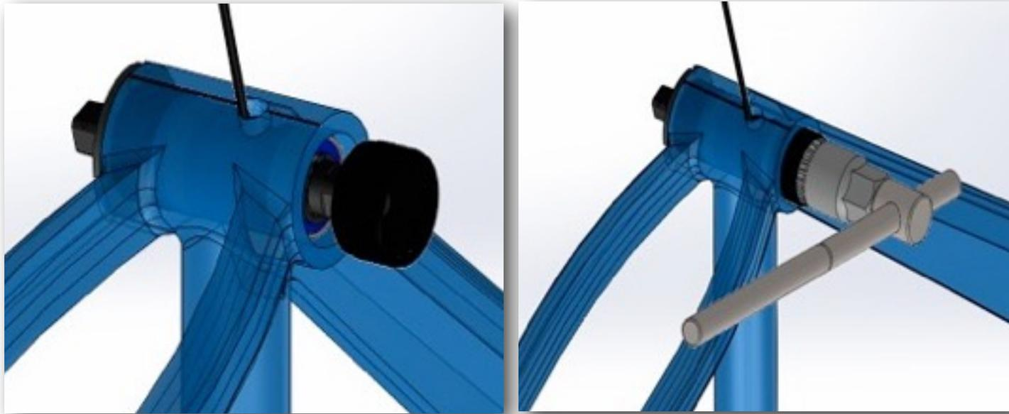
1. Screw the left side cup clockwise into the bottom bracket shell.
