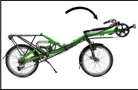
Bring right pedal to the front and fold handlebars forward
