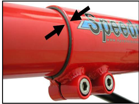
The plastic bushing between front boom and main frame must be visible at all time
