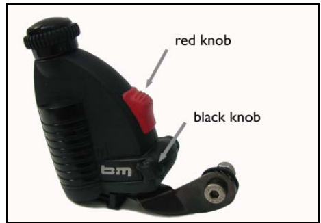
The tire dynamo has a red knob to turn it on. To turn it off it must be swivelled away from the tire.
