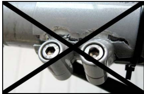
If there is no bushing or the bolts were tightened too fast, the front boom clamping might be damaged
