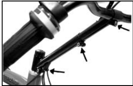
Clamping of the fixed stem with above seat steering
