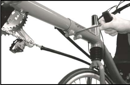
Loosen the clamping to adjust the length of the front boom.
