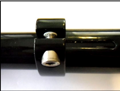
Clamping of the height adjustment for above seat steering. The end of the upper stem half must not be visible in the clamping slot.
