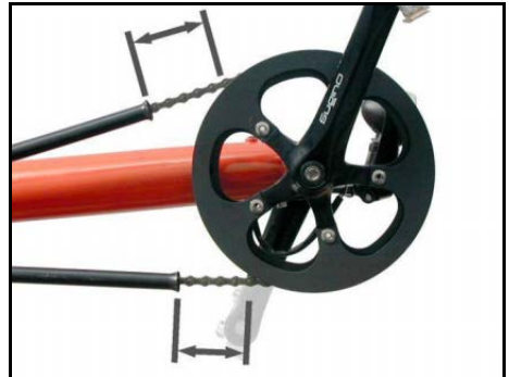
Check that there is at least a 5 cm (2") clearance between the end of the chain tube and other parts of the drive train.
