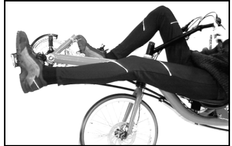
Adjust the front boom in a way that your knee will not be fully straightened when pedalling.
