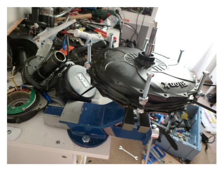
Then be patient and rise up the power on each screw step by step and please do it equably because otherwise the house become an angle and can destroy the Motor, You can see how the cover go apart:
