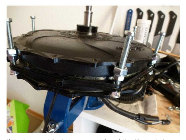
After ten minute you come to the point where you can separate the cover (cable-side) from the rest and now you have one Motor-cover in your hand and the motor with controller in your other hand:
