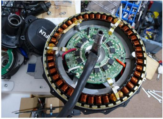
Now you can remove the controller by cutting the wires , we don't need the controller anymore because in our workshop we want build up a Bionx without Bionx electronic:
