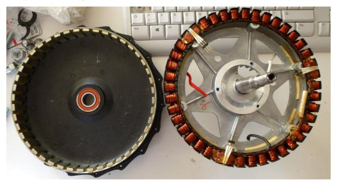
The Motor has 42pole and 43magnet
